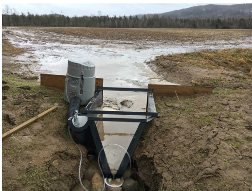
Figure 5. Flume capturing surface runoff during snowmelt event on 1/12/18 for tile-drained field, NNYADP Tile Drainage project, 2017.
