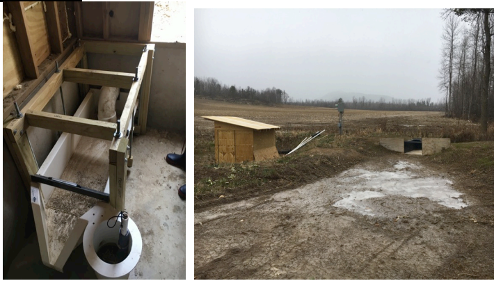
Figure 1 (left). Tile drain monitoring setup inside shed for tile-drained field, NNYADP Tile Drainage project, 2017.
