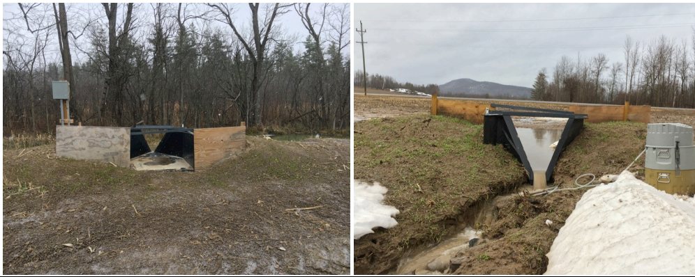
Figure 3 (left). Flume for measuring surface water runoff for undrained field, NNYADP Tile Drainage project, 2017.
