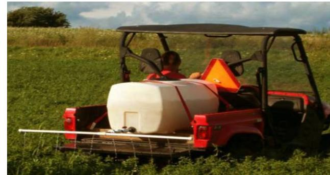
Gary Sullivan, Lewis County, sprays with a gravity feed sprayer made from PVC pipe.
