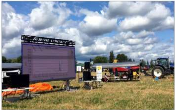
Below-ground soil pressures being measured under a tractor and baler and displayed in real-time at the Soil Compaction Field Day hosted by the Dundas Soil and Crop Improvement Association and the OMAFRA Soil Compaction Team in August 2019, near Inkerman, ON. Photo credit: K. O'Neil.
