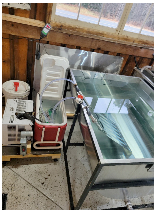
Figure 2: Left: the larger DIY chiller connected to the cooling plates on a 1500-gallon insulated dairy tank. These lines typically pump refrigerant through the cooling plate but glycol can be pumped through the plates. Right: the smaller DIY chiller connected to a cooling plate submerged into an open top tank.
