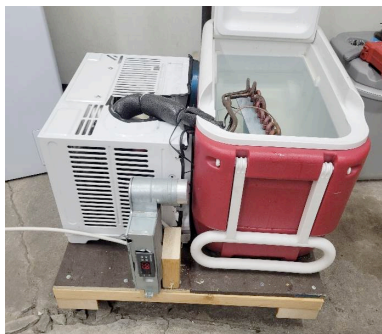
Figure 1: DIY glycol chilling unit made from a window AC unit and a plastic cooler. Cooling coil from front of AC unit immersed in glycol solution inside of cooler. New temperature controller installed within the aluminum box. The chiller unit sits on a wooden base with castor wheels for easy transport. Photo: Adam Wild
