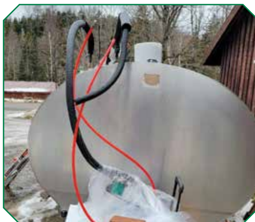
Above: DIY glycol chiller connected to cooling plates on 1,500-gallon insulated dairy tank.
