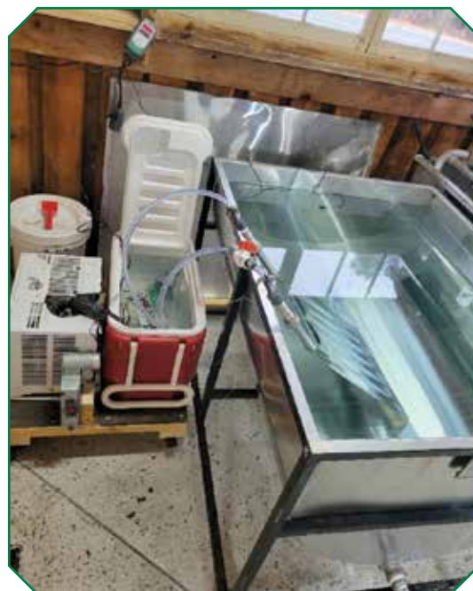
Above: DIY glycol chiller connected to cooling plates on 1,500-gallon insulated dairy tank.
