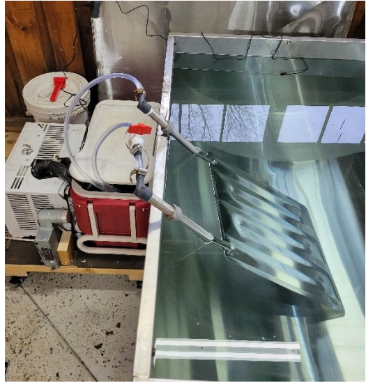
Figure 7. Cooling plate connected to glycol chiller submerged in tank of sap
