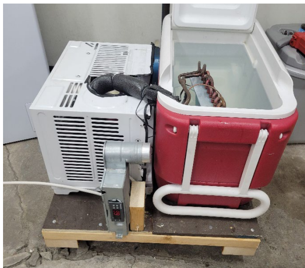
Figure 9. DIY glycol chilling unit made from a window AC unit and a plastic cooler. The chilling coil from the front of the AC unit is immersed in glycol solution held inside of the cooler. A new thermostat is installed within the aluminum box. The chiller unit sits on a wooden base with castor wheels for easy transport.
