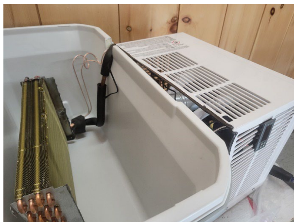
Figure 10. Outer housing and thermostat installed. Note where the housing meets up again the cooler it was trimmed back to fit closer. A cutting blade on an angle grinder was used to trim the metal. Electrical tape was used to cover the sharp metal edges after cutting.
