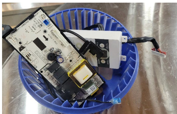
Figure 4. Thermostat on the front of the coiling coil (above). Components from the AC unit that are not needed: circuit board, thermostat, and blower wheel (below).
