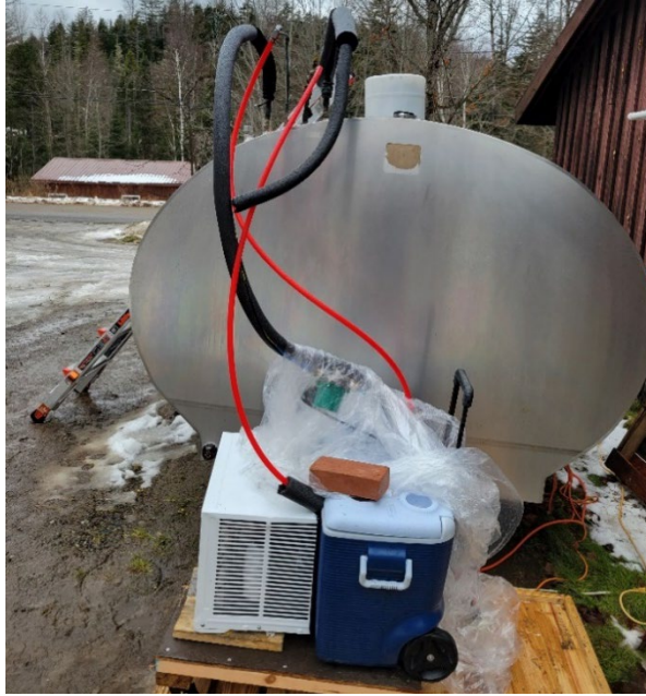
Figure 12. Left: Larger DIY chiller connected to cooling plates on a 1500-gallon insulated dairy tank. The lines were designed to pump refrigerant through the cooling plate, but here are used to pump glycol through the plates. Right: Smaller DIY chiller connected to a cooling plate submerged in an open-top sap tank. Chilled glycol is pumped from the chiller through the cooling plate and back. A temperature controller on the back wall measures the temperature of the liquid in the tank and turns the pump on and off when the set temperature is reached.
