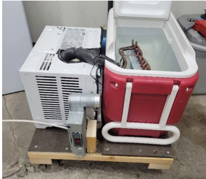
Figure 1. A DIY glycol chilling unit made from a window AC unit and a plastic cooler. The chilling coil from the front of the AC unit is immersed in glycol solution inside of the cooler. A new thermostat is installed within the aluminum box. The chiller unit sits on a wooden base with castor wheels for easy transport.
