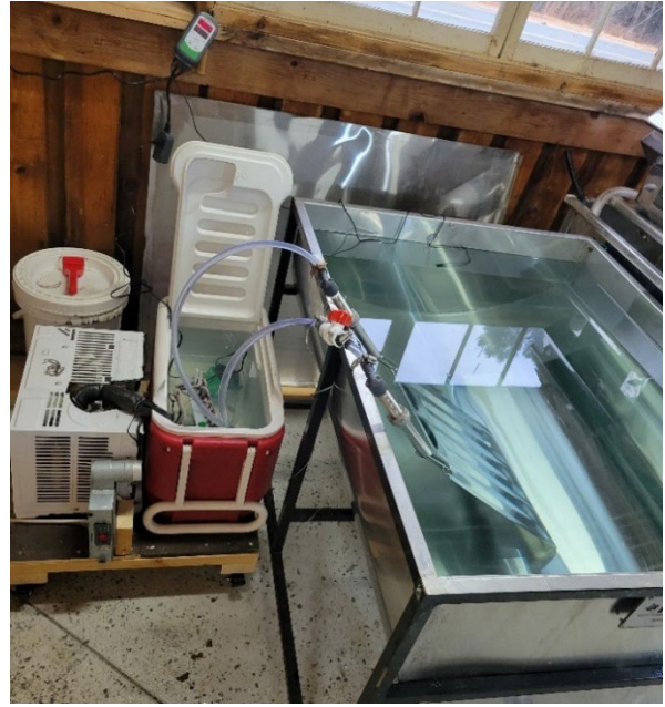
Figure 12. Left: Larger DIY chiller connected to cooling plates on a 1500-gallon insulated dairy tank. The lines were designed to pump refrigerant through the cooling plate, but here are used to pump glycol through the plates. Right: Smaller DIY chiller connected to a cooling plate submerged in an open-top sap tank. Chilled glycol is pumped from the chiller through the cooling plate and back. A temperature controller on the back wall measures the temperature of the liquid in the tank and turns the pump on and off when the set temperature is reached.
