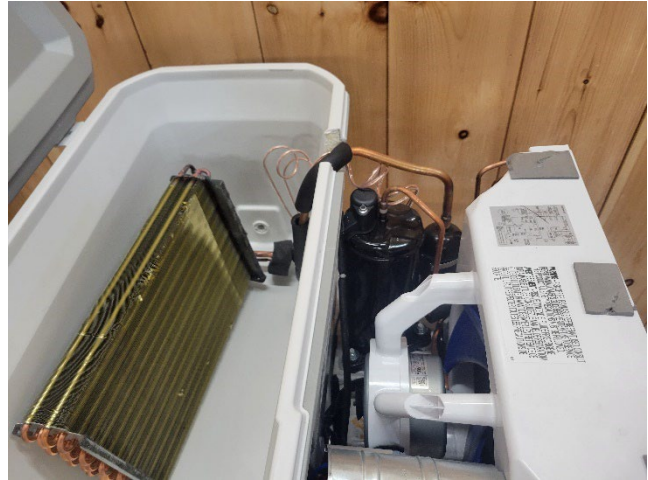
Figure 5. Chilling coil inserted into picnic cooler. Notice the notch in the top of the cooler for the copper lines to sit in while allowing the lid to close.
