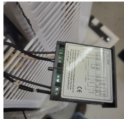
Figure 8. Wire diagram needed for powering AC unit through Inkbird ITC 1000 temperature controller.
