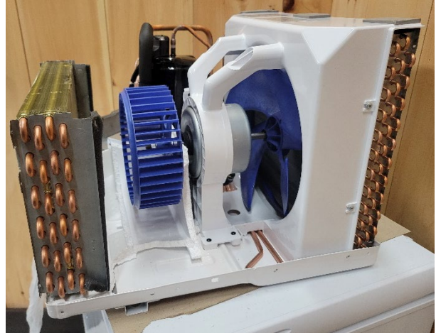
Figure 1. Window AC unit with outer housing removed. The chilling coil is the metal part on the far left with the curvy copper lines coming out of it. To the right, of the chilling coil, you can see the blue blower fan. The black tower behind the blower fan is the compressor. The blue blade fan further to the right is the cooling fan. On the far right with more curvy copper lines coming out is the condensing coil.
