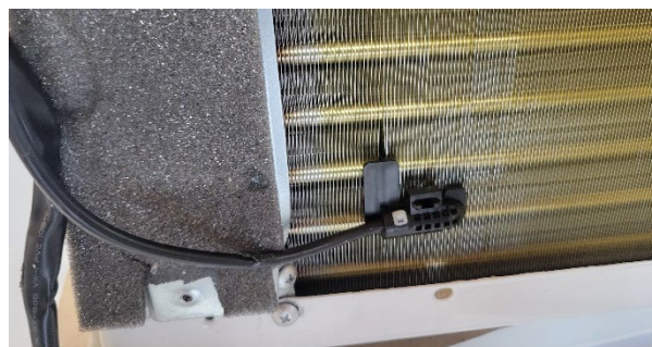
Figure 4. Thermostat on the front of the coiling coil (above). Components from the AC unit that are not needed: circuit board, thermostat, and blower wheel (below).
